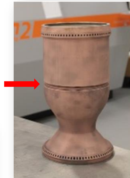
Sections Stacked; Mid-section weld & EBF 3 Applied
