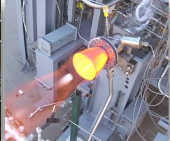
C-CAT Extension Test, ZrB2/HfC EMCC
