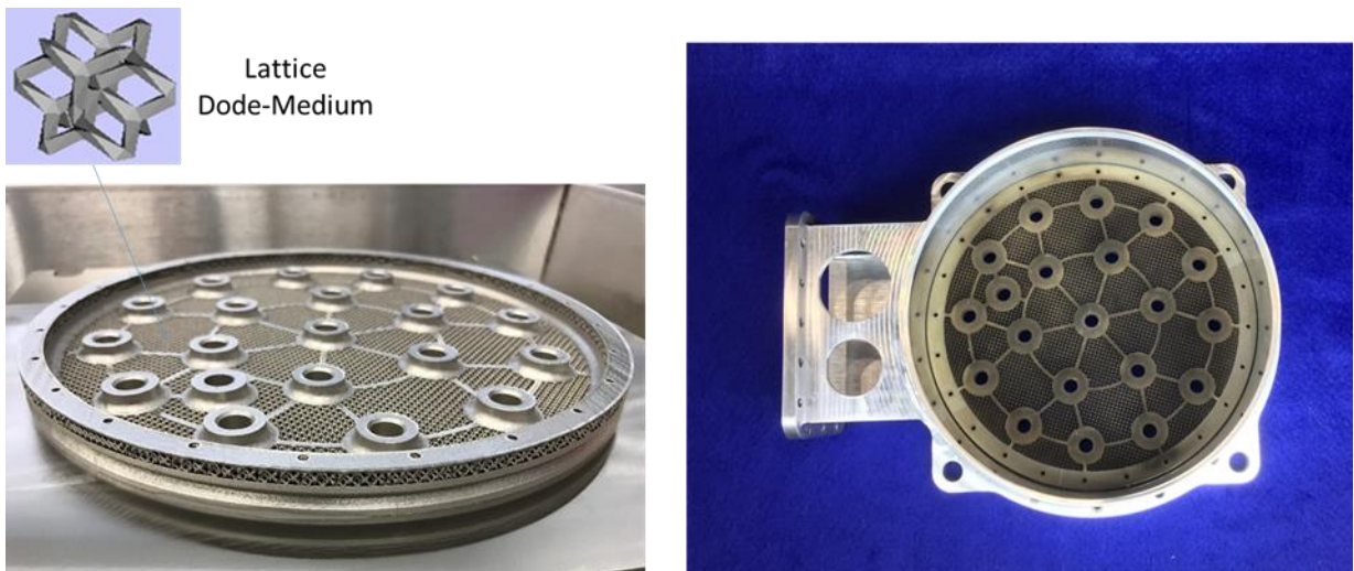
Figure 4. 4BMS-X Heater Mounting Plate and Sorbent End Cap
