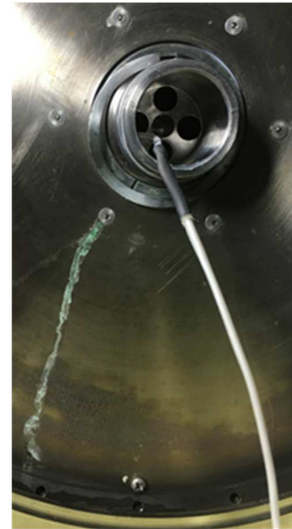
Figure 2. Pretreated urine leak through a bearing of the DA.
