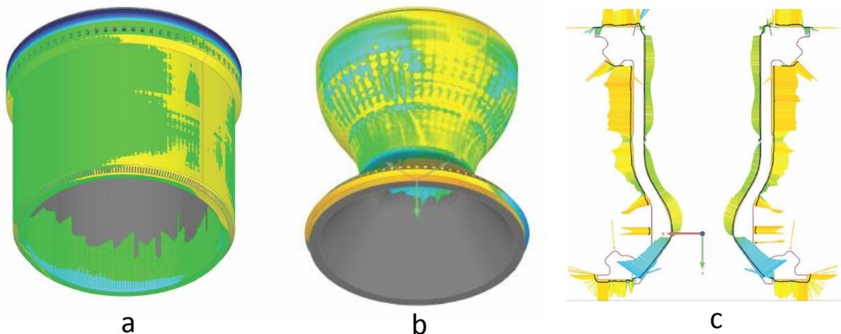
**Figure 12. (a) Structured light scans of post SLM, post HIP chamber halves, (b) post-EBF3 deposition and post HIP joined unit and (c) 2D cross section of post-EBF3 deposition.**
