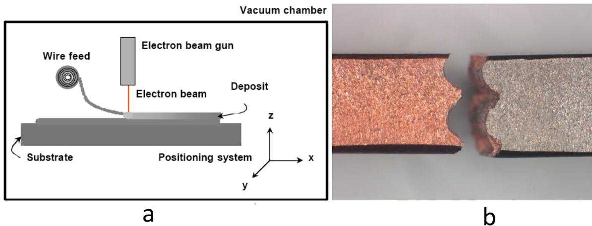
**Figure 10. (a) EBF<sup>3</sup> Process and (b) Pull test specimen after test to failure on the GRCop-84 to EBF<sup>3</sup> Inconel 625 bond interface.**
