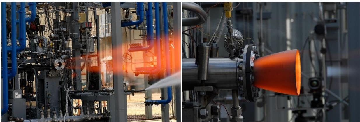
**Figure 29. Hot-fire testing of the GRCop-84 additively manufactured liner with the stainless slip jacket and Carbon-Carbon nozzle extension<sup>27</sup>. The chamber accumulated a total of 2,365 seconds of hot-fire time. [Photo credit: David Olive/MSFC]**
