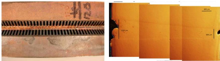
**Figure 14. Chamber Halves Joint Trial EB Weld.**
