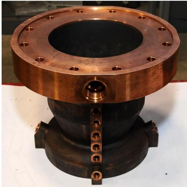
**Figure 17. Methane Cooled SLM GRCop-84 Throat Section Chamber.**
