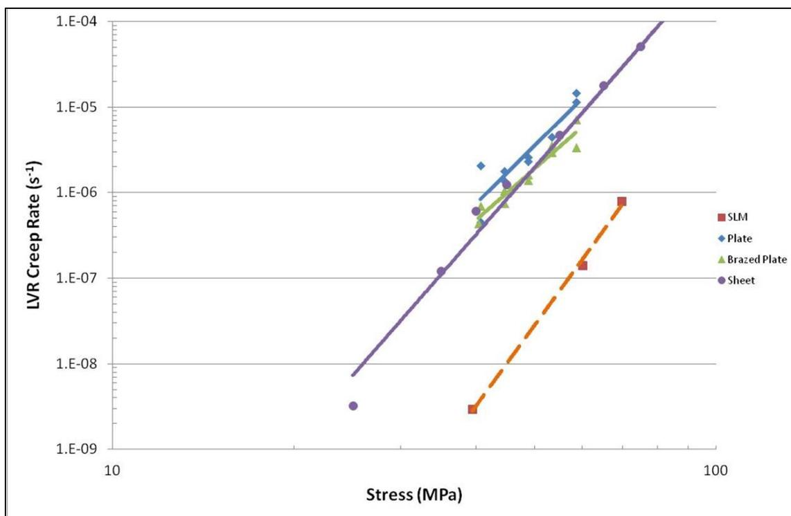
**Figure 6. 650 °C (1472 °F) Creep Rate of Conventionally Processed and SLM GRCop-84.**
