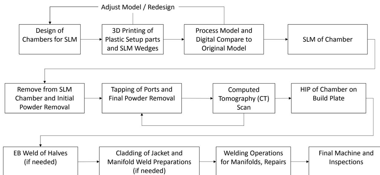
**Figure 30. Generic process flow for Design and Fabrication of SLM GRCop-84 chambers.**
