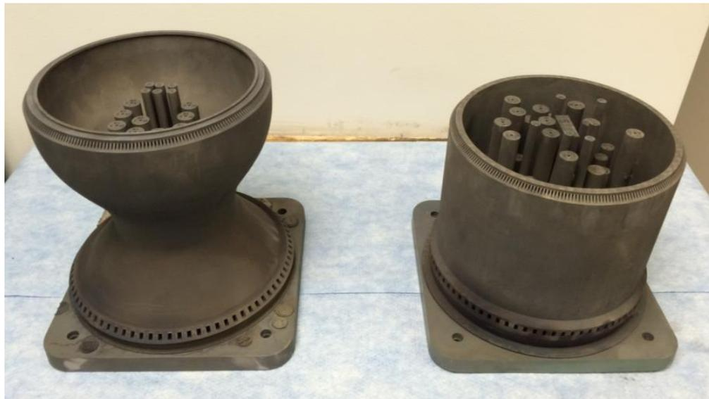
**Figure 8. 3D Printed Chamber Sections for LCUSP.**
