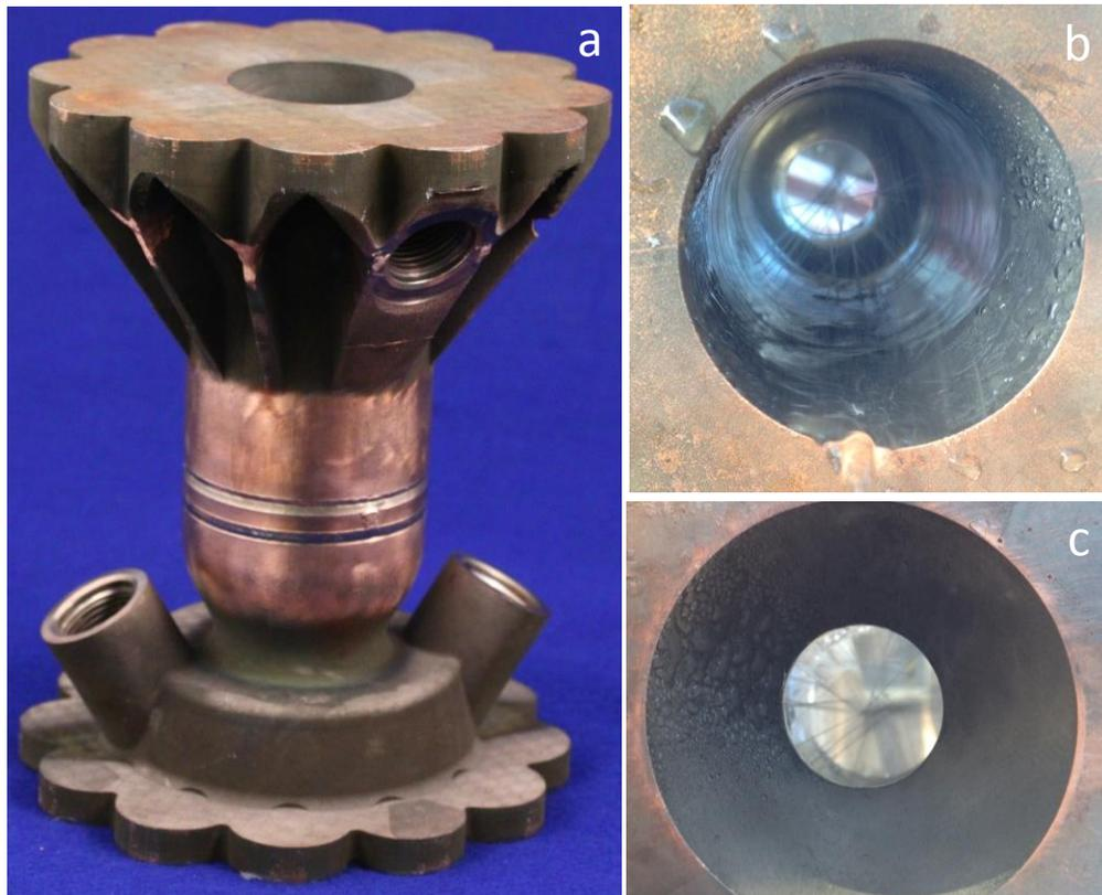
**Figure 25. Completed 1.2K One-piece chamber: a) Completed chamber with EB weld of split ring and repairs of cracks, b) pinhole leaks during water flow from forward end, c) Pinhole leaks as seen from aft end in the area of the EB weld split ring.**
