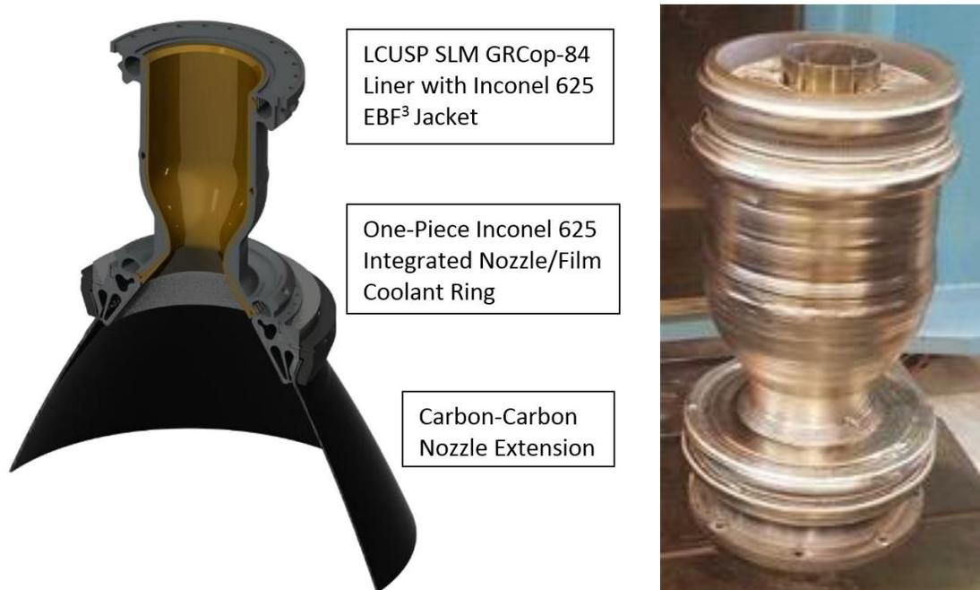
**Figure 7.(a) LCUSP Thrust Chamber Assembly and (b) Hot Fire Test Article after joining and EBF<sup>3</sup> Deposition – Image (b) Courtesy Karen Taminger**
