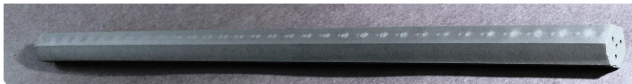
Figure 1 Oakridge Fuel Element Tested in NTREES to Meet the NCPS Milestone
