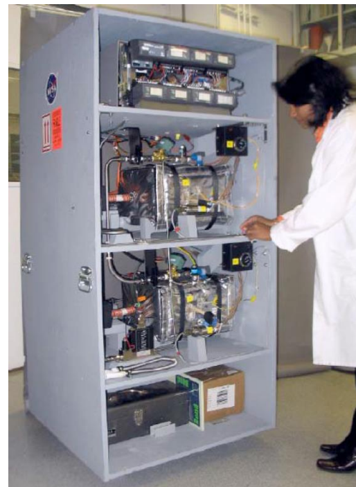
Figure 8. AC-TSAC Undergoing Preparation for the Integrated Atmosphere Revitalization Tests 34
