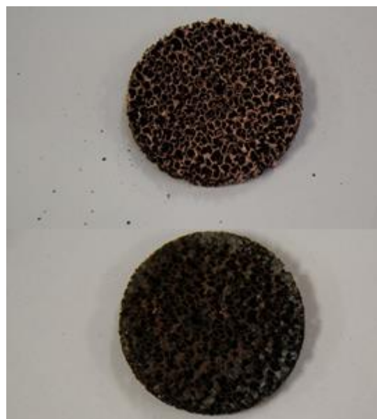
Figure 2. Fe-plated Cu puck post carbon regeneration (above) and the regenerated Fe-plated Cu puck after electroplating (below).
