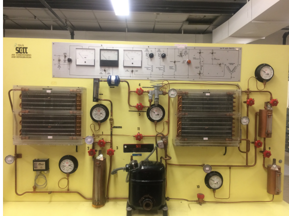
Figure 4. Vapor Compression Laboratory Demonstration, University of Utah Department of Mechanical Engineering
