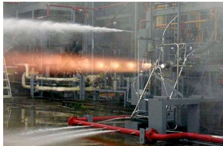
Hot-fire test of GRCop-84 Liner, image from: Loewenthal, William & Ellis, David. Fabrication of GRCop-84 Rocket Thrust Chambers . Slide 16
