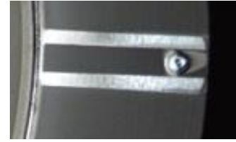
Figure 6. Mo strip on OFPC with graphite mask.
