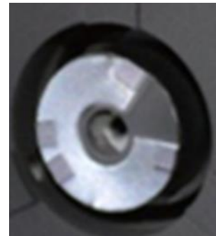
Figure 4. Mo mask on keeper electrode.
