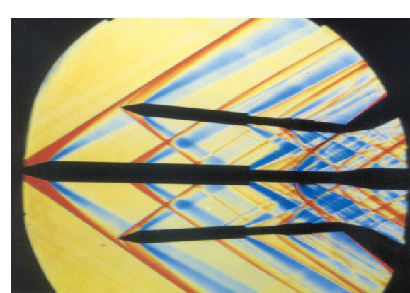
Schlieren flow-visualization of booster separation
