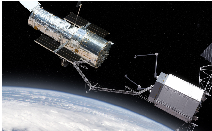
Figure 4. A first-generation TALISMAN supporting autonomous in-space servicing.
