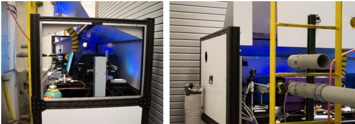
Figure 3. Laser cart. Left: back of the cart. Right: Front of the cart with the two beams being shot through the tubes.
