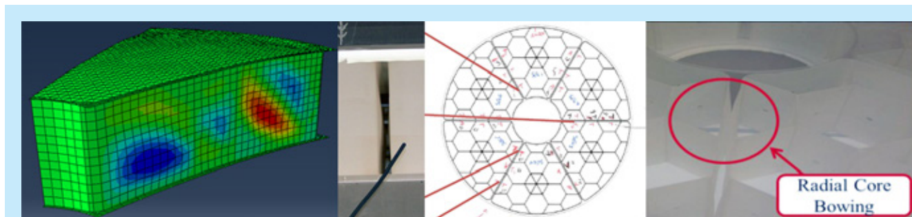
Fig. 2. Left: predicted visco-elastic deformation used to design mirror substrate. Center Left to Right (3 images): actual visco-elastic deformation; four locations had gaps of less than 0.25 mm.
