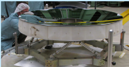
Fig. 3. Coated 1.5-m ULE® AMTD-2 mirror.
