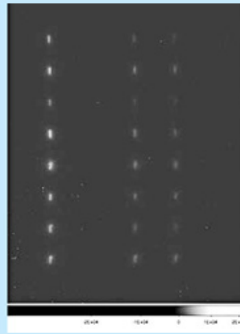
Fig. 4. Left: Delta-doped and AR-Coated EMCCD (CCD201), optimized for 200 nm, in the dewar at Palomar's CWI. Right: CCD in FIREBall spectrometer with Zn lines around 200 nm indicating good performance for FIREBall's atmospheric window at 205 nm.
