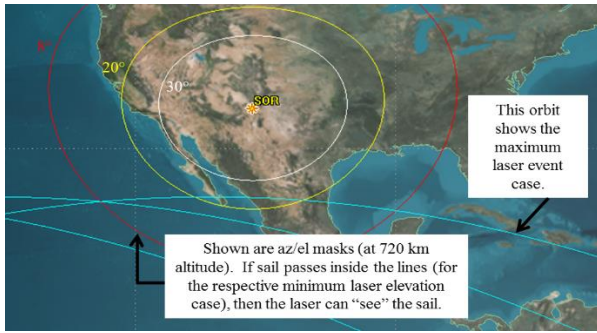
Figure 2. The LightSail 2 can only be engaged by the SOR laser at low elevation, likely violating range safety requirements.
