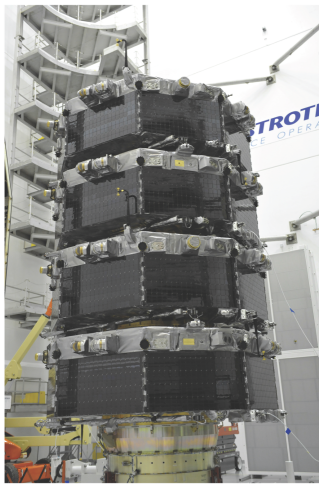
Figure 3: Stacked launch configuration of the four MMS spacecraft. The GPS antennas can be seen as black dots at each of the corners of the instrument deck (credit [13]).
