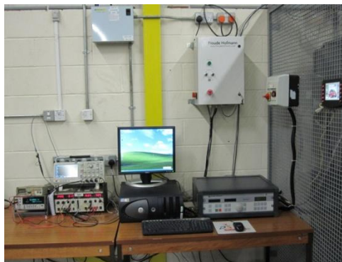
Fig.3. Dynamometer control and datalogging equipment
