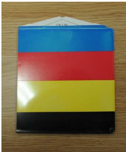
Figure 6 Photograph of the dye sublimation decorated component
