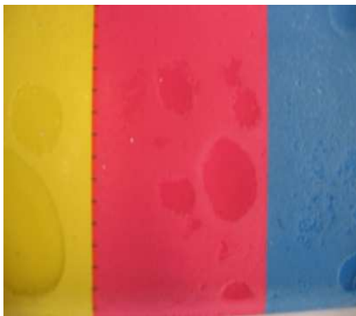
Figure 28 PC Photograph of the surface showing thermal damage
