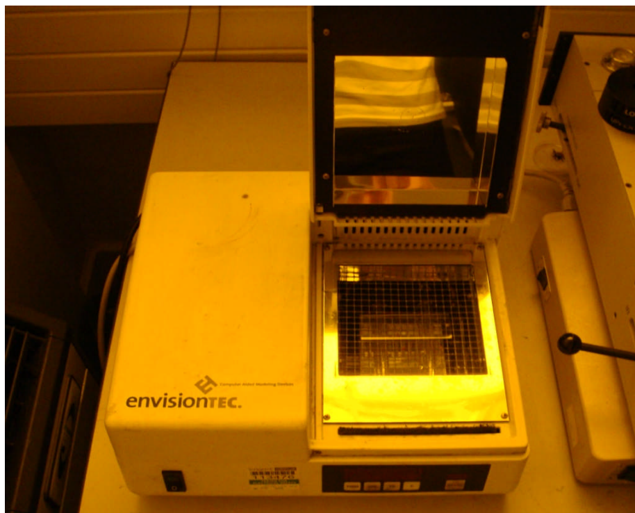
Figure 4.8: The Otoplast post-cured flash box for post-curing processes
