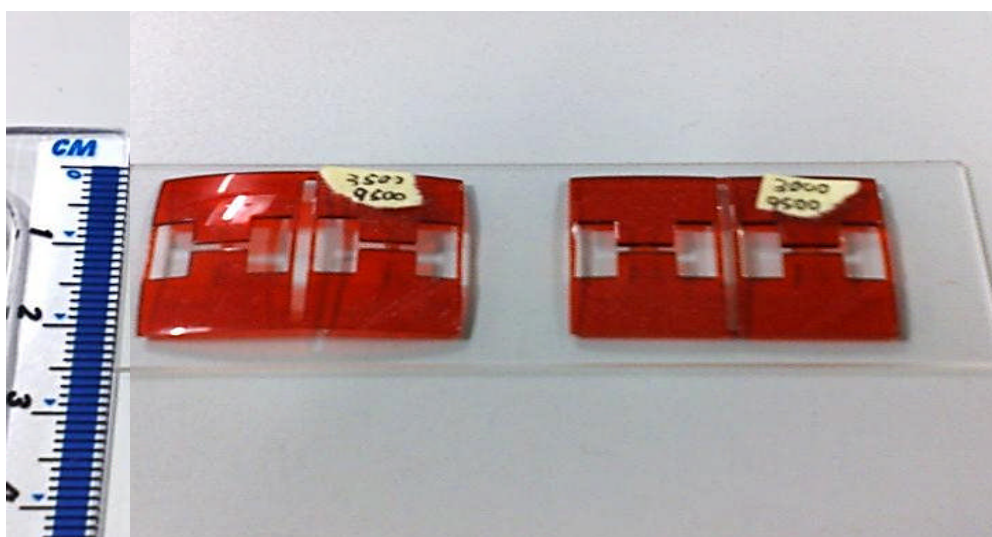
Figure 4.16: Specimens (1 mm thickness) with 3.5 and 3.0 s UV exposure (left: 3.5 and 9.5 s curing; right: 3.0 and 9.5 s curing)
