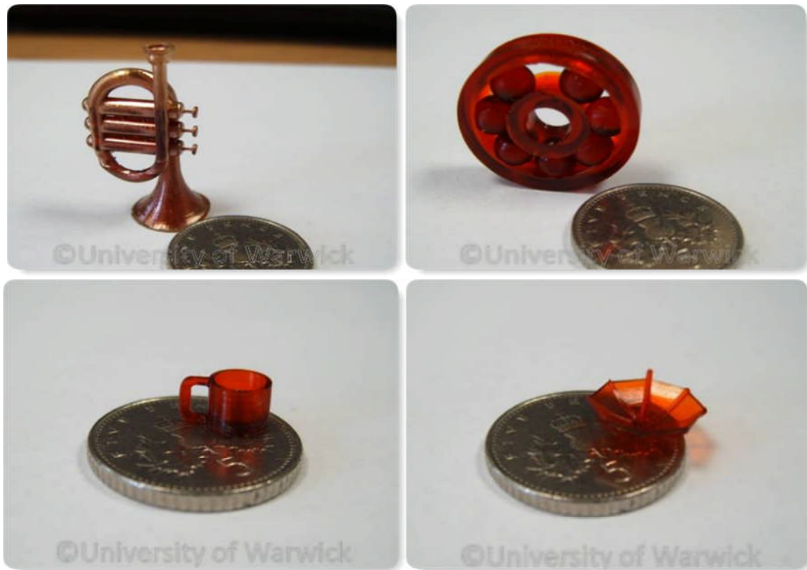
Figure 4.2: Small objects fabricated in resin R11 on a 5p coin for scale (Leigh, 2010)
