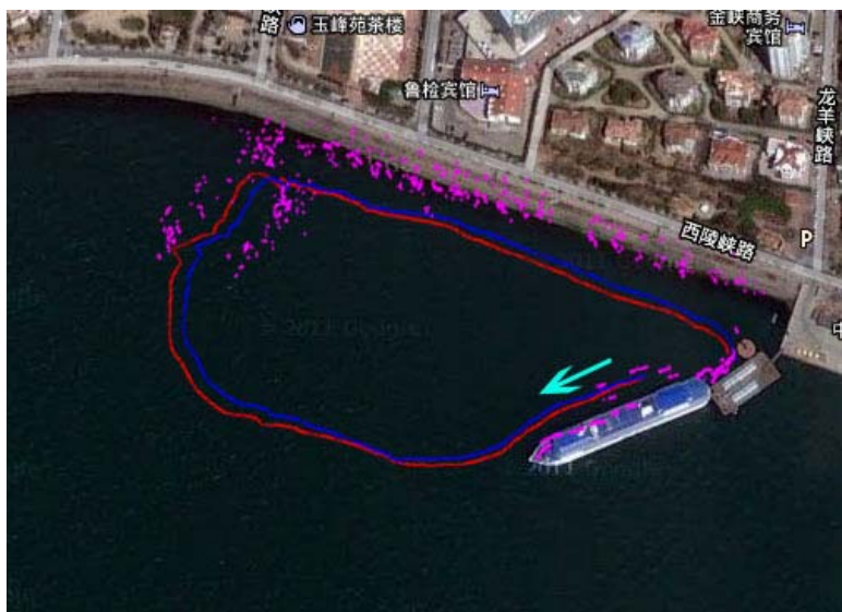
Figure 11. The modified FastSLAM resulting map combined with the environmental map.
