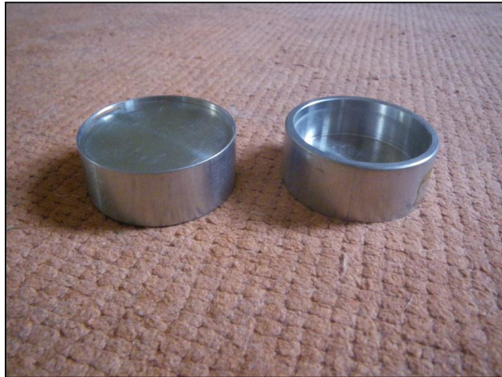
Figure 2.2: Two contact corers. The left hand contact corer is upside down showing the sample skirt area. The right hand core is upright and shows the well for liquid nitrogen.
