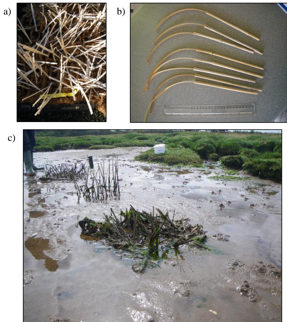
Figure 7.1: Biodegradable seagrass mimics; a) reed and coir mesh, b) reed on bamboo anchors, and c) test plots in the Tay estuary.
