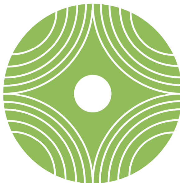
Figure 37. SynRM with axially laminated rotor [23].
