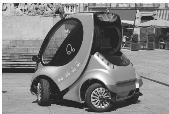
Figure 14. Hiriko Fold—a vehicle employing in-wheel motors.
