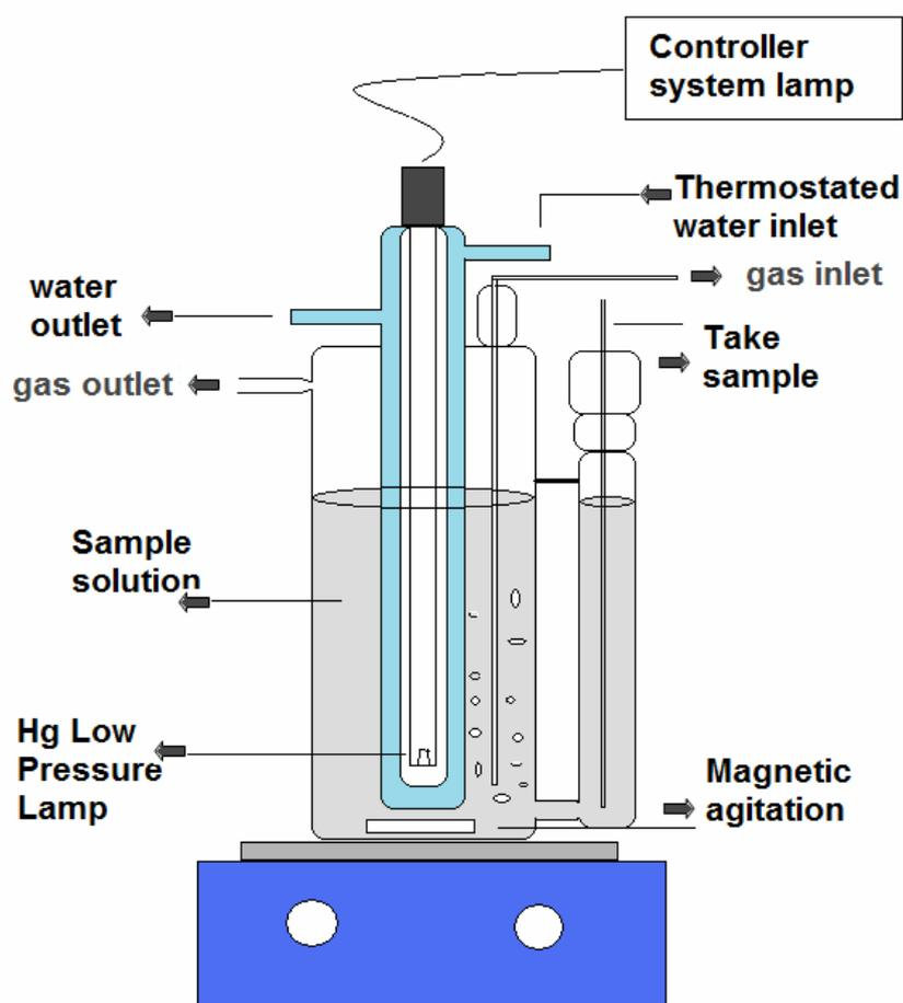
Figure 19. Photodegradation Instrument
