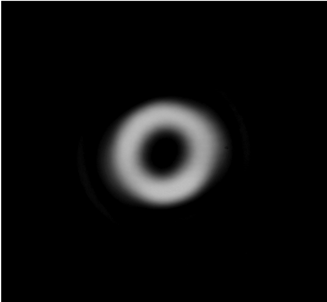
Figure 2.12: Image of the transverse profile of the Pump Beam Diffracted by the computer generated hologram. The image has been captured via an high sensitivity CCD camera. It is evident the hole in the middle, distinctive of the higher order Laguerre-Gaussian modes. The characteristics of the hologram allows for the generation of intense LG_{02} modes.
