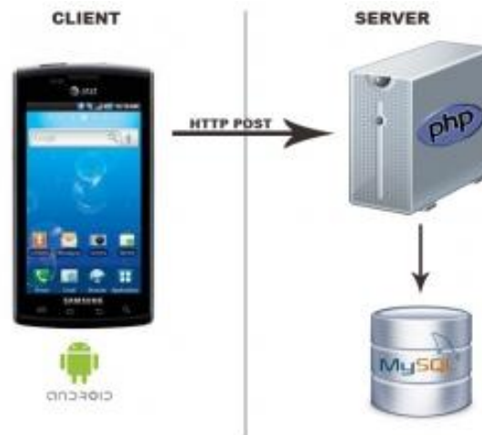
Figure 2 Connection between PHP (server) and Android (client) using HTTP and JSON ( http://fahmirahman.wordpress.com/2011/04/21/connection-between-php-server-and-android-client-using-http-and-json/ )
