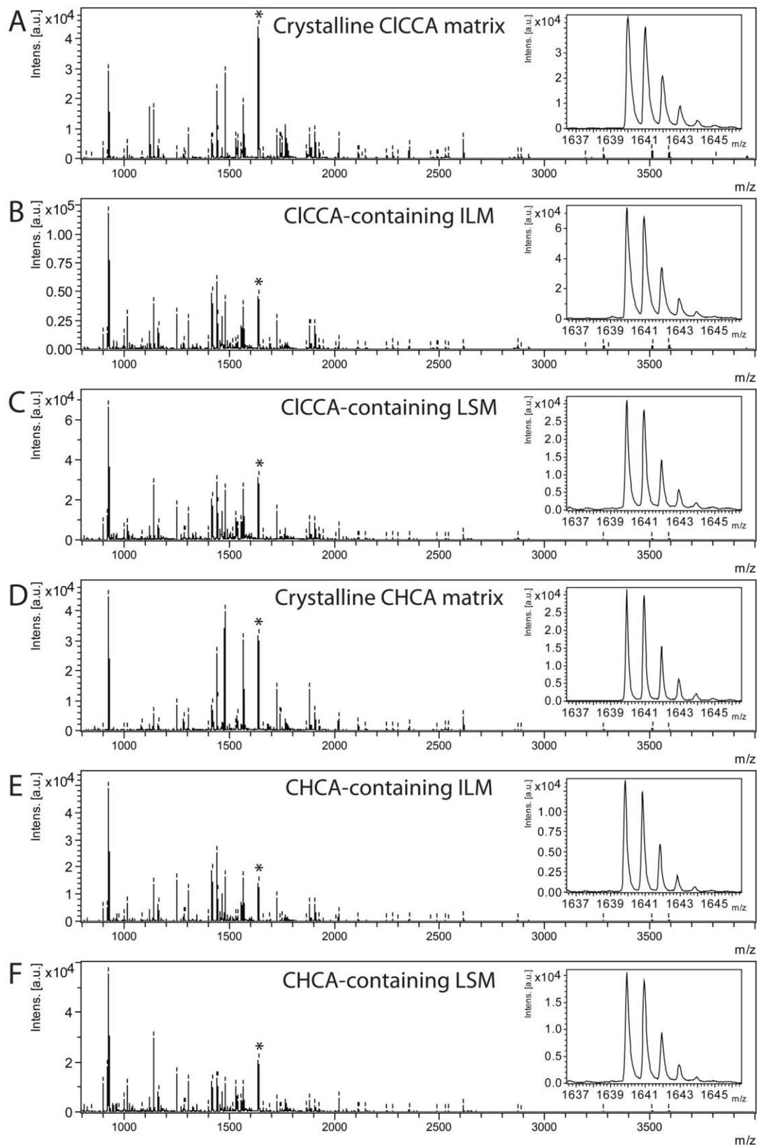
Figure 5. Example mass spectra of an in-solution BSA digest with 100 fmol spotted on target for (A) crystalline C1CCA matrix, (B) C1CCA-containing ILM, (C) C1CCA-containing LSM, (D) crystalline CHCA matrix, (E) CHCA-containing ILM and (F) CHCA-containing LSM. A total of 500 single-shot spectra were acquired per spectrum. Tick-marks denote peaks matching theoretical BSA tryptic digest masses. \* denotes expanded peak.
