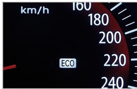
Figure 2.1: Kia’s driving system is using a coloured lamp to indicate the energy-efficiency of the driving behaviour [16]
