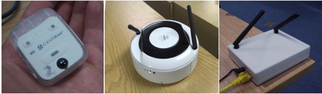
Figure 6.1: RTLS hardware components used in this study: Tag, Monitor, Star
