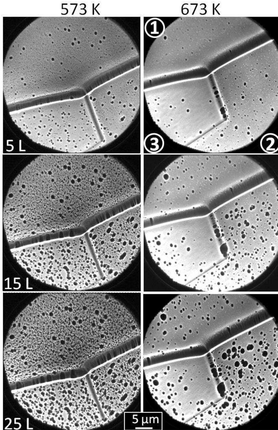
FIG. 4: LEEM images (MEM mode) recorded during the oxidation of polycrystalline Ni at  $1 \times 10^{-8}$  mbar of oxygen. Left column: exposure at 573 K to 5, 15, and 25 L; right column: exposure at 673 K to 5, 15, and 25 L. The region shown here is outside the area mapped in Figure 1; the orientations of the three facets (1), (2), (3), indicated in the top right image, have not been identified by micro-spot LEED.
