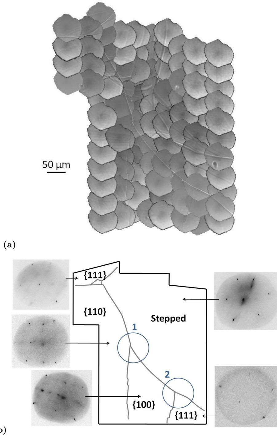
FIG. 1: (a) Surface map (area  $500 \times 750 \mu\text{m}^2$ ) compiled from LEEM (MEM) images of  $80 \mu\text{m}$  field of view showing five adjacent facets. **(The distorted image boundaries are due to the profile of the electron beam.)** The boundaries between the facets are indicated in the schematic drawing in the center (b); the additional lines seen in the map of (a) on the stepped facet in are scratch marks; micro-spot LEED patterns of each facet are also shown in (b).
