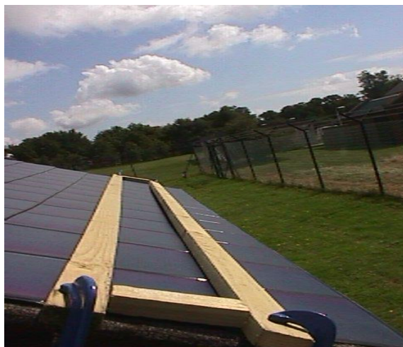
Figure 13 Shading 3a-Si with battens
