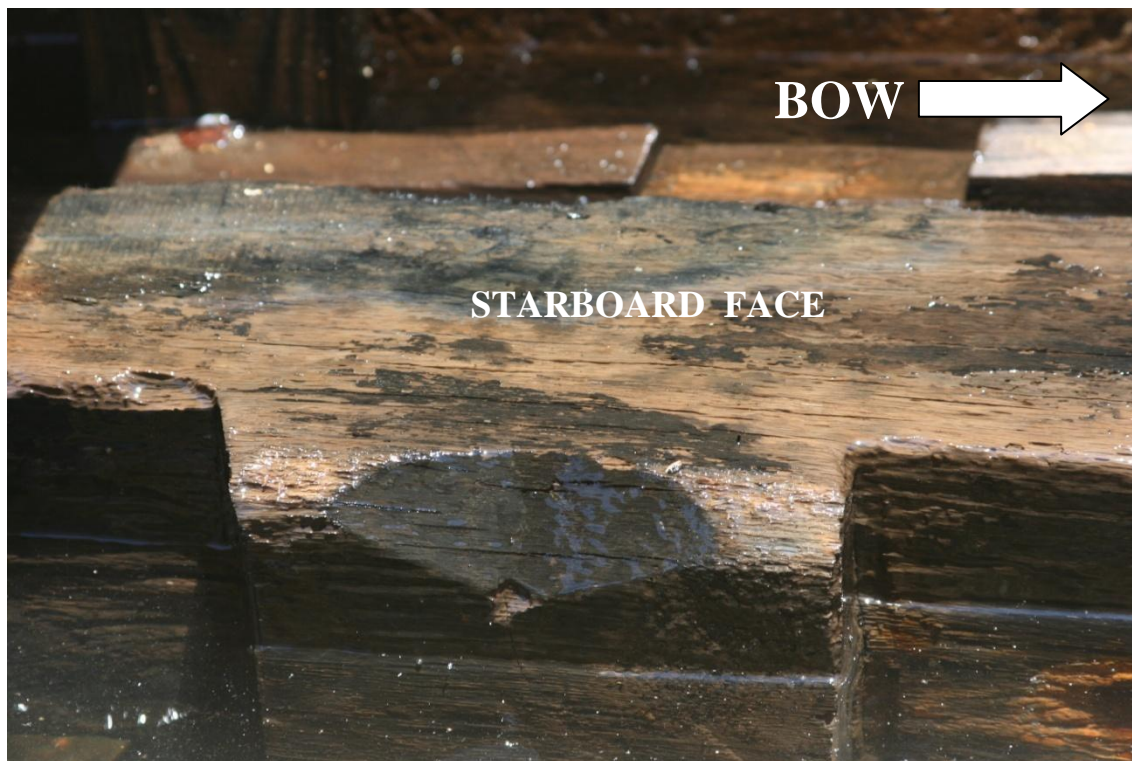
Figure 4.51: Wood between the notches showing reverse-triangle or chevron-shaped finish.
