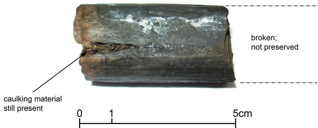
Figure 4.10: Example of a partly preserved treenail with a V-shaped caulking cut and caulking material.
