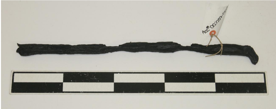
Figure 4.7: Preserved section of a wrought iron bolt with clenched tip (00:057-009) (one scale unit equals 10 cm).
