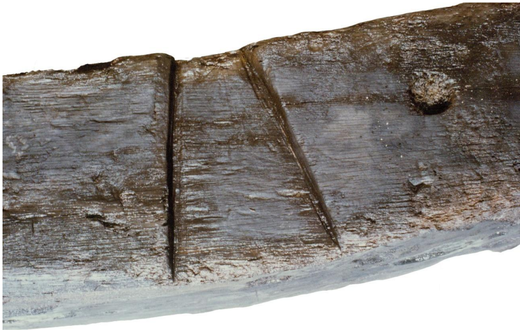
Figure 4.28: Example of the dovetail mortise on the port side of floor timber A. (FR A)
