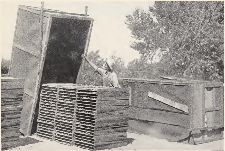
Fig. 2. The hood-type sulfuring equipment, shown above, may be lifted over stacks of trays. It is of temporary construction, but may be used in a small operation, or to supplement other equipment.
