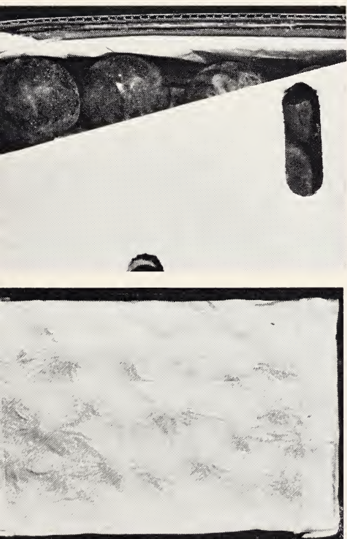
Fig. 17. Above, top: Cutaway view of pad in position over top fruit in container. Slight pressure of lidding holds pad firmly against fruit.
