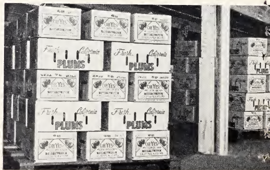
Fig. 24. Tight-fill plum containers stacked on pallets for cooling. Note cross stacking and spacing of containers.
