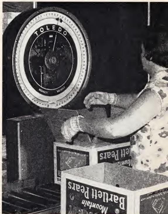
Fig. 9. Check weighing of filled containers before vibration settling. Clear view of scale dial speeds this operation.
