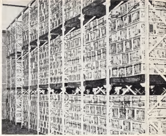
Fig. 25. Tight-fill packed pears in storage in permanent pallet racks. In this system, each pallet is independent of all others.
