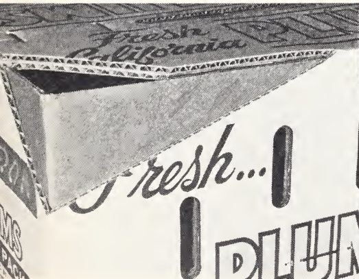
Fig. 20. Cutaway view of corrugated container showing the lid tightly seated against the rim of the body. Tight seating is necessary to maintain the tight-fill pack and thereby avoid fruit injury resulting from movement during subsequent handling.
