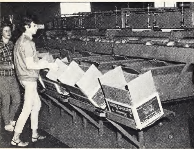
Fig. 6. Above: Table being used to assemble containers for automatic filling. After assembly, pads are placed in lids and containers are filled while inverted.
