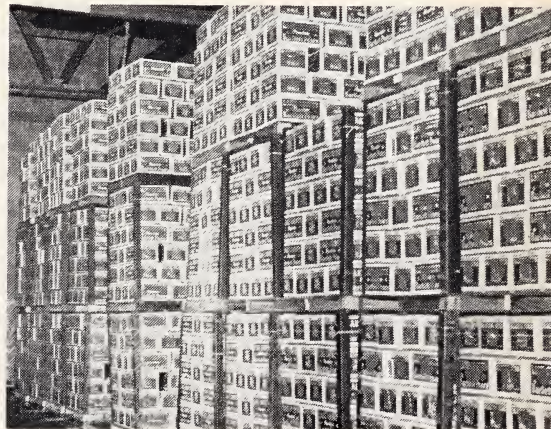
Fig. 26. Pallet supports of "crutches" being used for tight-fill pear storage. The corner supports carry the weight of top pallets.
