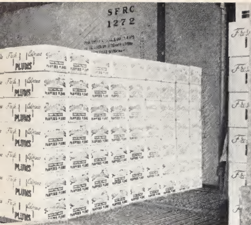
Fig. 27. Tight-fill packed plums loaded solid in a rail car. This method is suitable only for thoroughly cooled fruits with a fairly low respiration rate.
