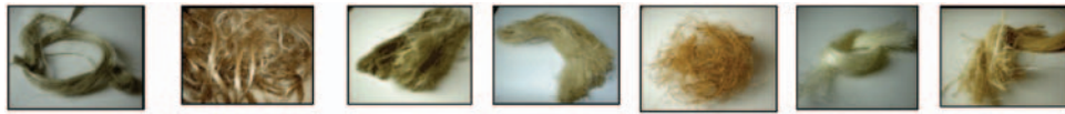
Figure 2. From left to right, flax, jute, kenaf, hemp, coir, sisal, and abaca.
