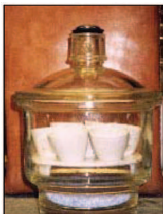
Figure 4. A desiccator similar to that used for controlling humidity.
