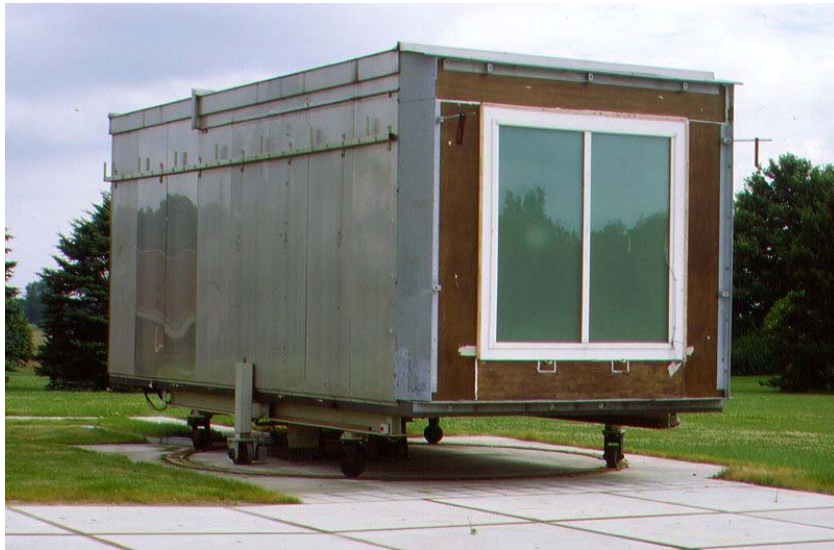
Figure 1: Advanced glazing component mounted on PASLINK test cell
