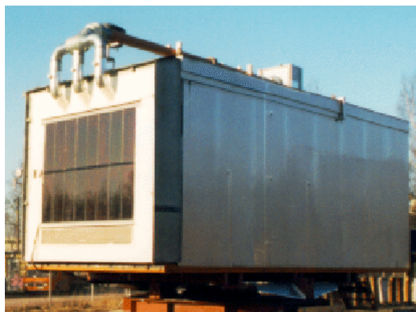
Figure 16: Ventilated PV-panel wall at the PASLINK test cell at VTT test site in Espoo, Finland
