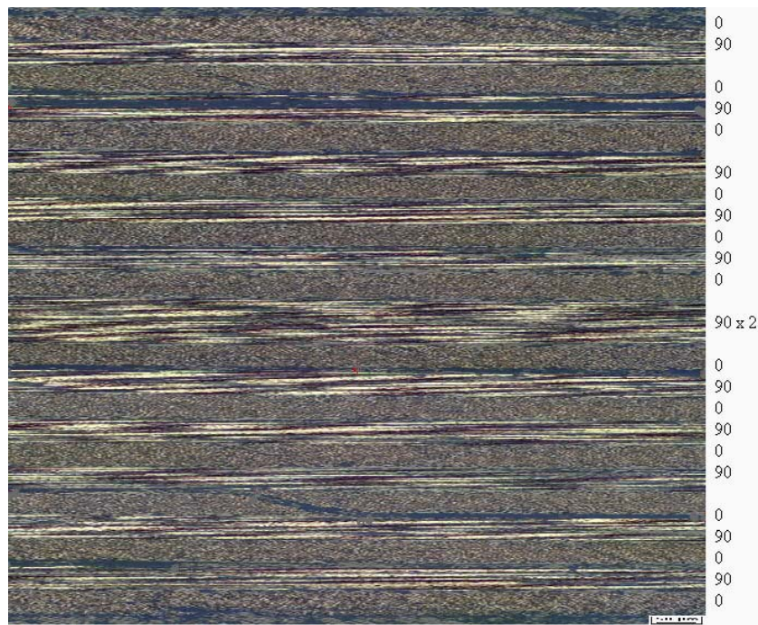
Fig 15b Micro-photographic image of through the impact face section of the second [0/90]_{6s} laminate.
