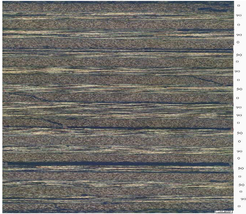
Fig 15a Micro-photographic image of through the impact face section of the first [0/90]_{6s} laminate..
