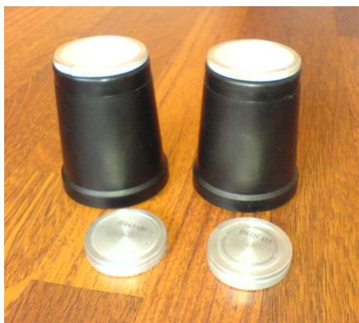
Fig. 1 Electret ion chamber detectors (200 ml volume)
