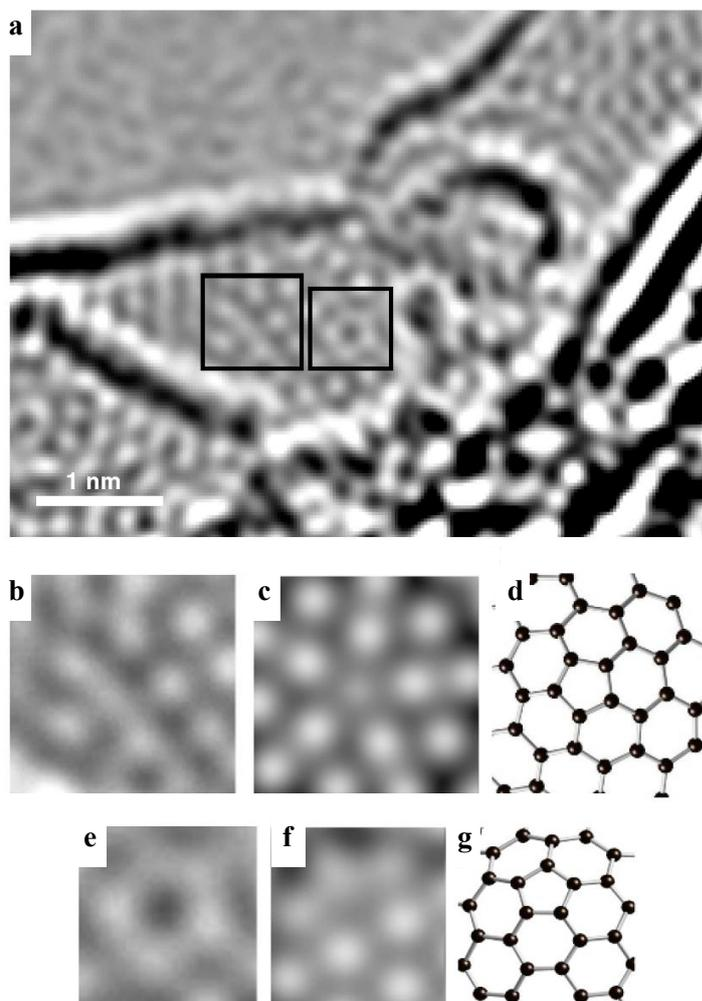
**Figure 4:** (a) Aberration-corrected micrograph of small area of the 2000°C-heated carbon. (b) Enlarged region showing pentagonal arrangement of spots. (c) Simulated image of structure shown in (d). (e) Second region showing pentagonal arrangement. (f) Simulated image of structure shown in (g).
