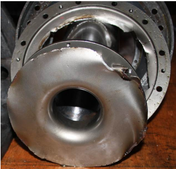
Figure 35. Angular Misalignment Failure
