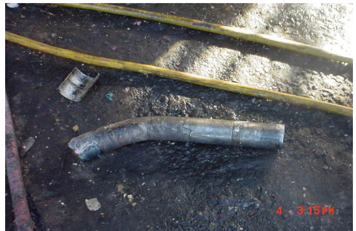
Figure 16. Section of Turbine Shaft
