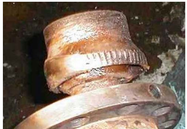
Figure 60. Heavy wear due to grease being displaced by water.
