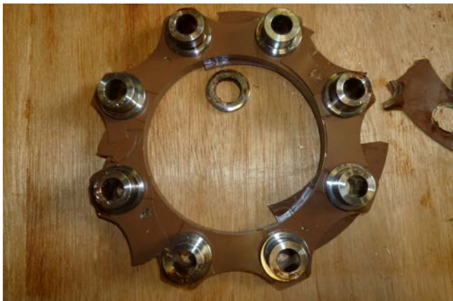
Figure 30. Disc Angular Misalignment Failure
