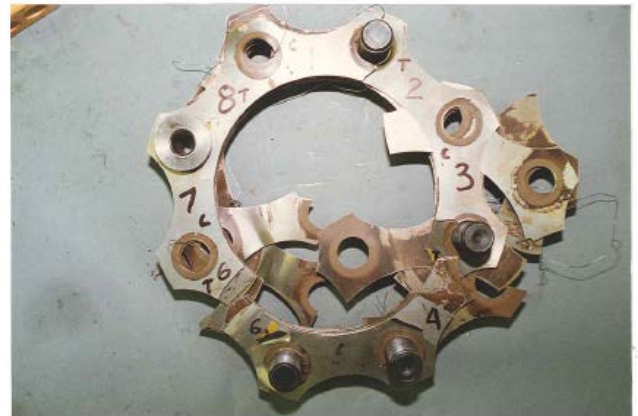
Figure 26. Failed Turbine End Discs
