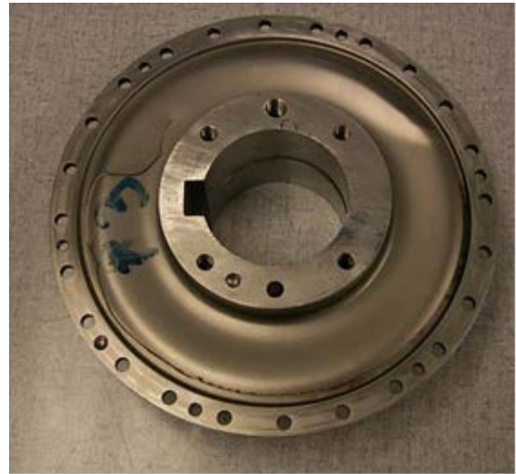
Figure 10. Excessive Angular Misalignment and Axial Movement Diaphragm Failure
