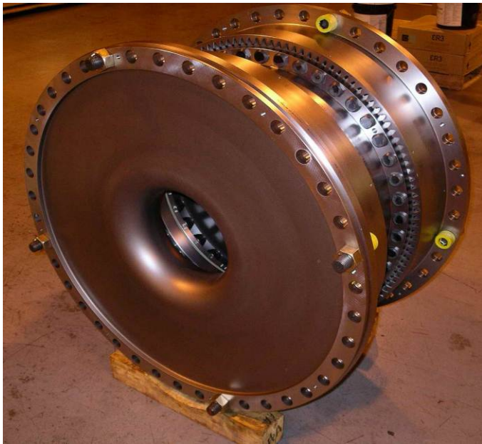
Figure 1. Special Purpose Diaphragm Coupling
