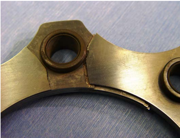
Figure 58. Failing disc pack with missing shards found by an alert operating crew!
