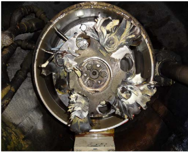
Figure 40. Disc Packs Ripped from Tremendous Forces
