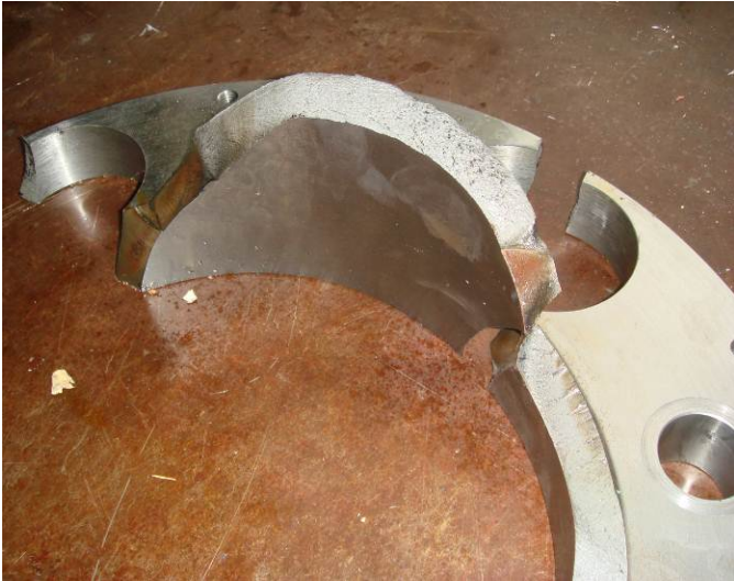
Figure 9. Excessive Torsional Oscillation Fatigue Failure in Spacer
