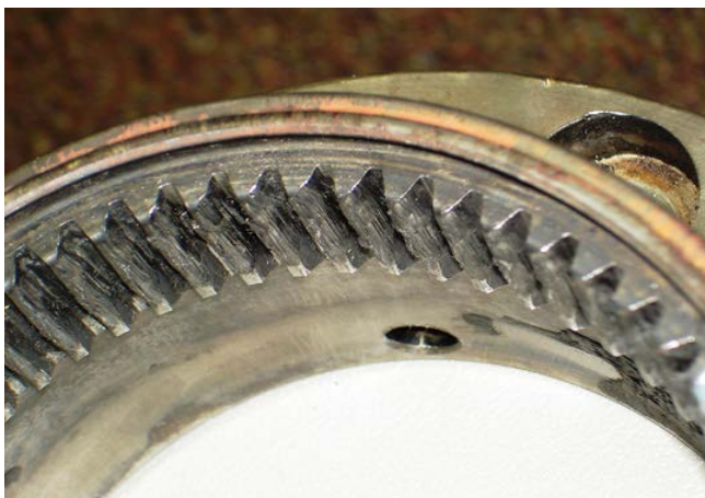
Figure 25. Heavy tooth scoring from loss of lubrication.
