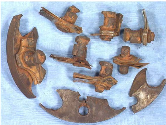
Figure 51. Remnants of compressor side disc pack & hardware
