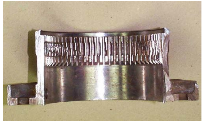
Figure 45. Coupling half, sectioned for easier viewing.
