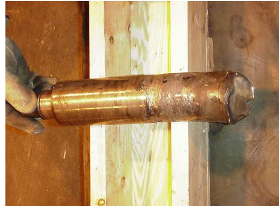
Figure 20. Opposite End of Failed Turbine Shaft
