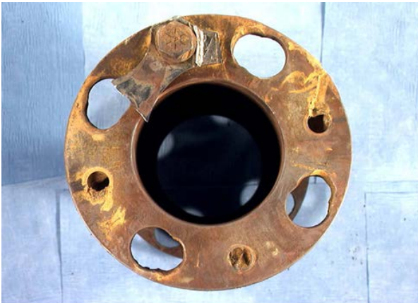
Figure 50. Oblong bolt holes in spool hub on compressor side.
