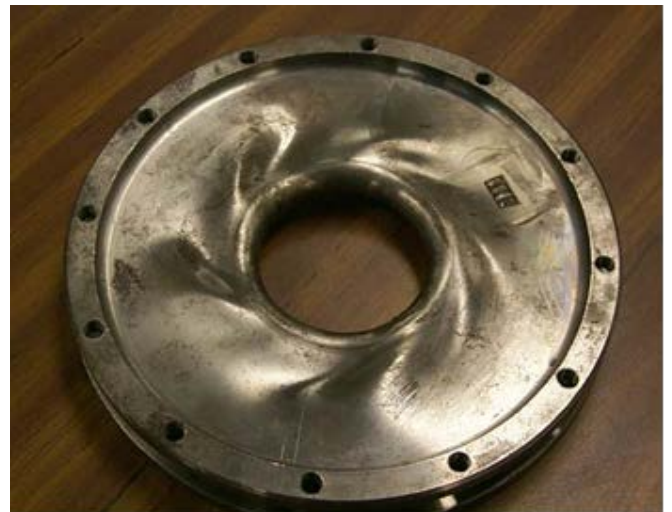
Figure 11. Diaphragm Torque Overload
