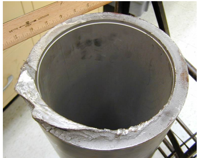
Figure 34. End of Spacer Tube; Failure Initiation Site is at 10 O'clock Position on the ID
