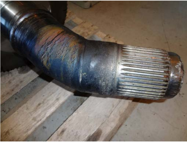
Figure 39. Bent Shaft from Heat
