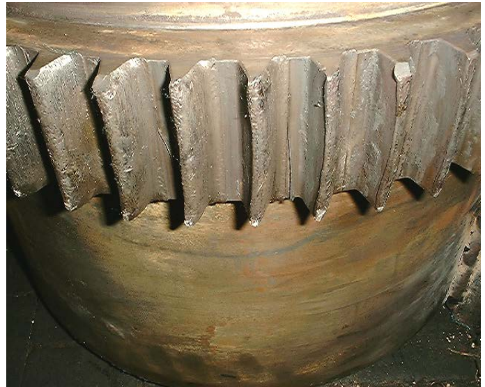
Figure 4. Gear Teeth Worn From Excessive Misalignment
