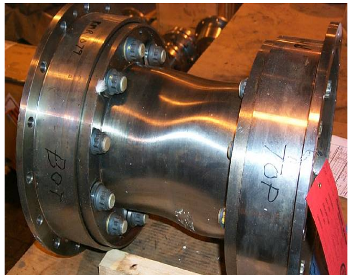
Figure 8. "Twisted Sister" Yielded (Buckled) Spacer From Over Torque
