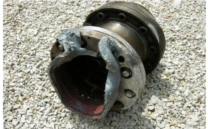
Figure 23. Friction heated coupling spool.
