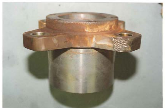
Figure 27. Interlock Engagement Wear on Hub
