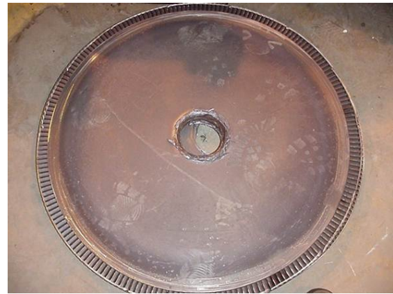
Figure 18. Turbine Disc with Damage at Bore
