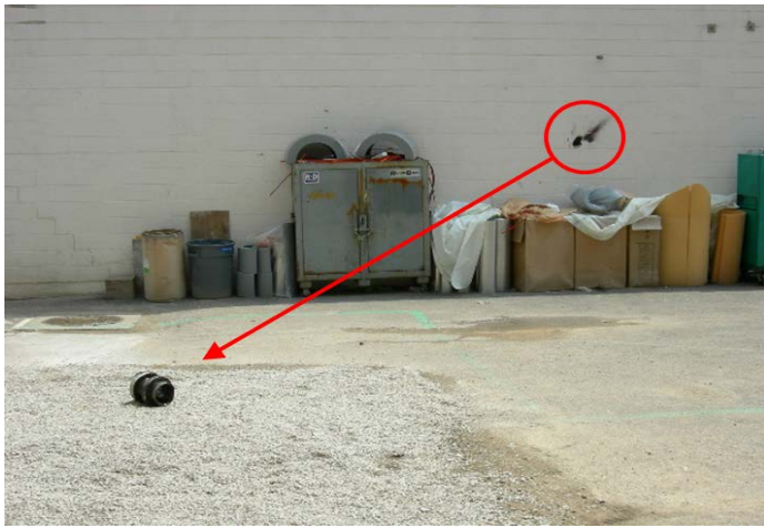
Figure 24. Ejected spool impact and final location.
