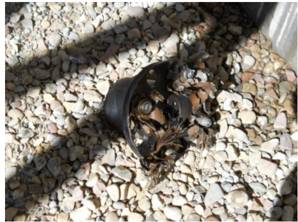
Figure 37. Hub with Disc Pack Ejection
