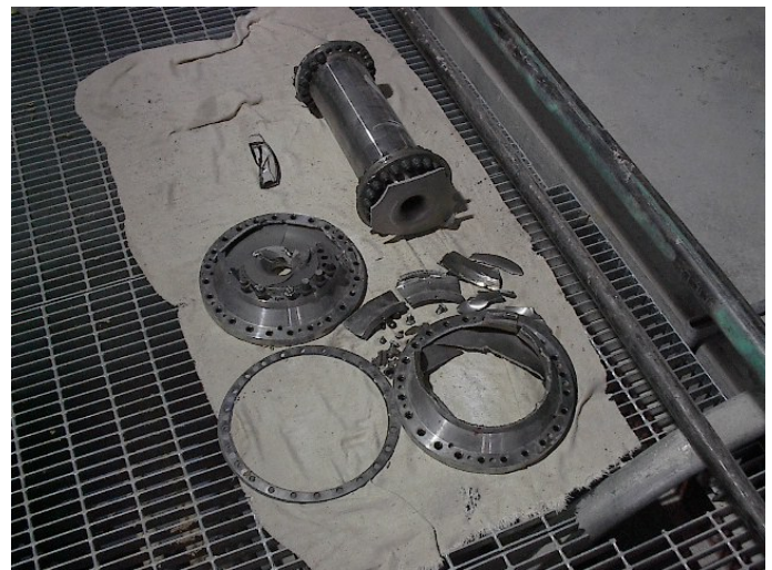
Figure 42. Ejected Parts when Anti-Flail did Not Work
