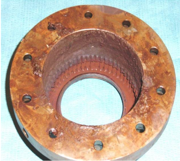
Figure 2. Excessively Worn Gear Teeth
