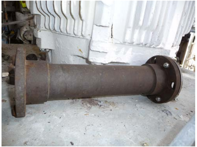
Figure 55. Disc pack spool piece was ejected on start up.
