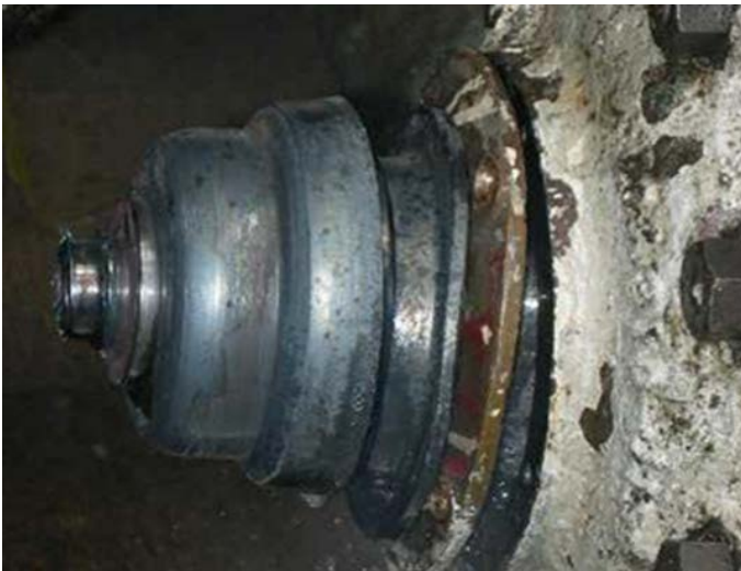
Figure 22. Friction heated coupling hub, teeth are gone!
