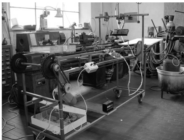
Figure 3: Test bench for flaming treatments in warm season turfgrasses.
