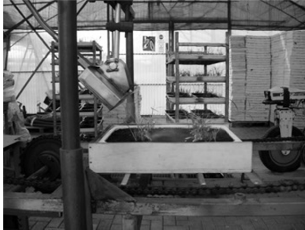
Figure 1: Test bench flaming treatment performed on a tray containing four warm season turfgrasses plants.
