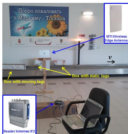
Fig. 2. Measurement setup at Grosseto Airport to validate the new technique for discriminating moving tags along a conveyor belt from static and nomad tags in a rich multipath environment.
