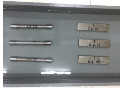
FIGURE 2: Specimens immersed in soil solution.
