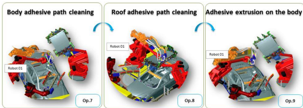
Figure 7.6. Automated assembly first steps [1]
