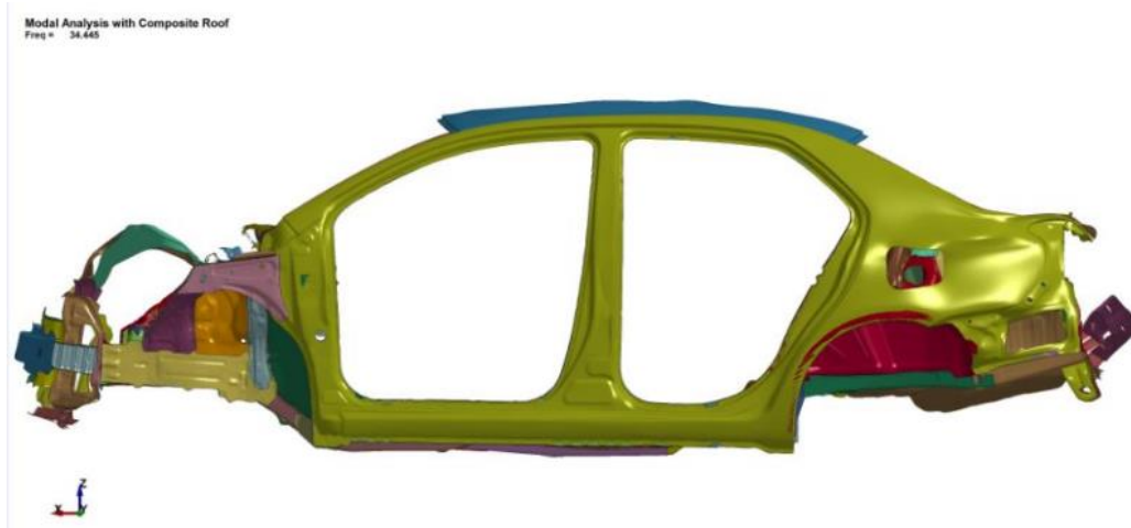
Figure 4.31: Chassis with steel roof first bending mode –34.4 Hz
