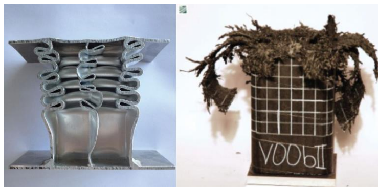
Figure 3.13: Comparison of metallic specimen folding and composite specimen fracture [4]
