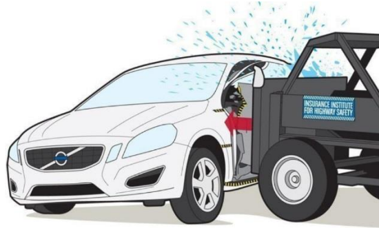
Figure 3.7: Schematic of side crash test
