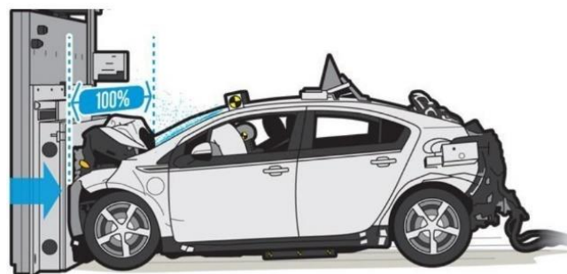
Figure 3.4: Schematic of full frontal crash test
