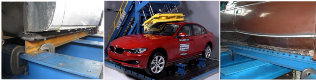
Figure 6.32: FMVSS 216 experimental test configuration [2]
