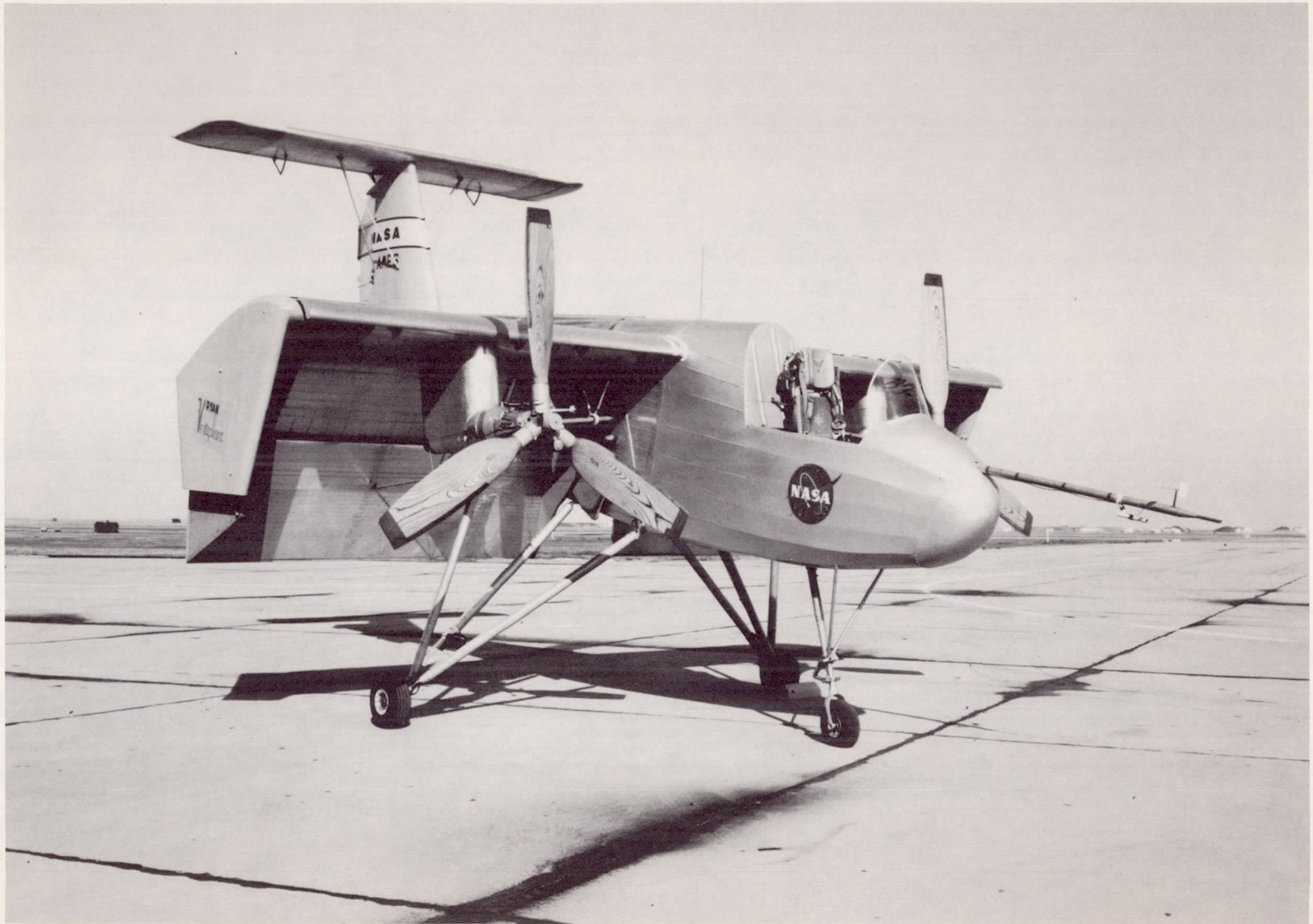
Figure 1.- The Ryan VZ-3RY deflected-slipstream test vehicle shown with leading-edge slat installed and with fully extended flaps.
