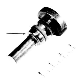
FIGURE 8 WATER-COOLED INSULATOR, ARROW INDICATES AREA WHERE PITTING CORROSION CAUSED LEAKS
