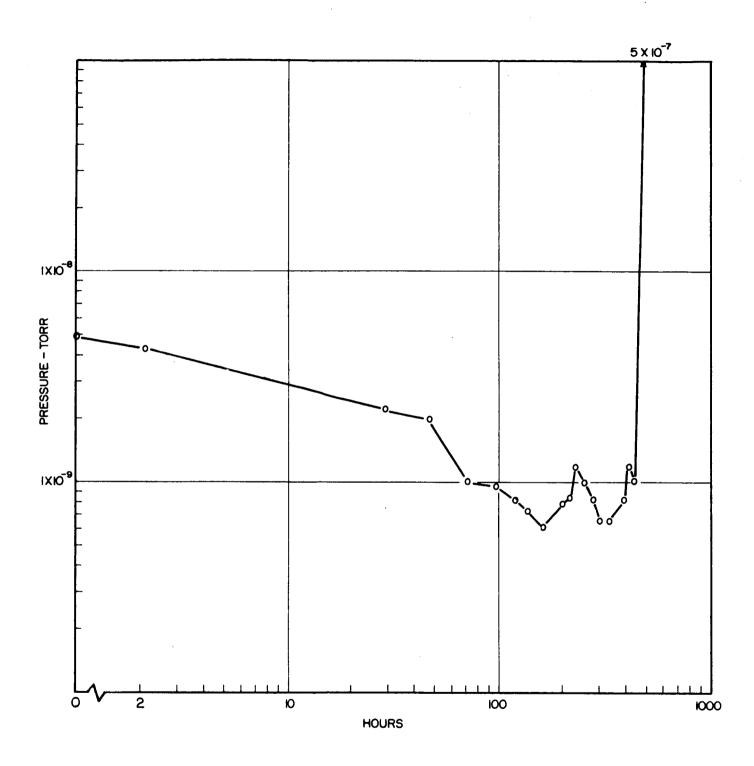
VARIATION OF VACUUM WITH TIME FOR TEST NO. 2 COLUMBIUM ALLOY, FS-85 2000°F, 7000 PSI.
