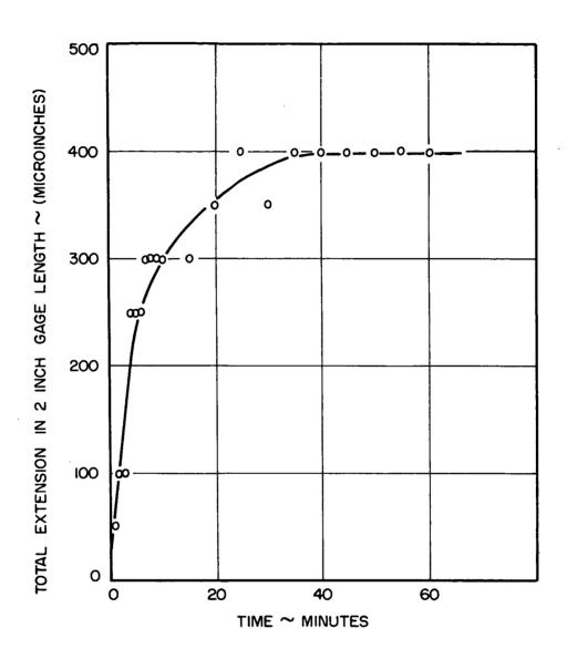
CREEP DATA, TEST NO. 2 COLUMBIUM ALLOY FS-85, 2000°F, 7000 PSI, < 10<sup>-8</sup> TORR, ONE HOUR PRIOR ANNEAL AT 2600° F.
