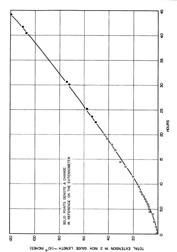
CREEP DATA, TUNGSTEN - 25% RHENIUM, 3200°F, 5000 PSI < 10- TORR, 48 HOUR ANNEAL AT 3200°F PRIOR TO LOAD APPLICATION.
