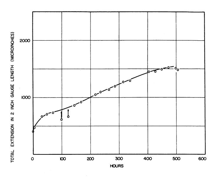
CREEP DATA, TEST NO. 2 COLUMBIUM ALLOY FS-85, 2000° F, 7000 PSI,  $< 10^{-8}$  TORR, ONE HOUR PRIOR ANNEAL AT 2600° F.
