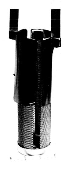
FIGURE 12 TUNGSTEN MESH HEATING ELEMENT WITH TANTALUM RADIATION SHIELDS ATTACHED TO IMPROVE GRADIENT
