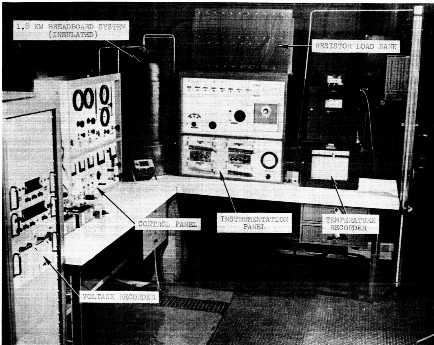
1.8 KW Breadboard System Test Setup Figure 5
