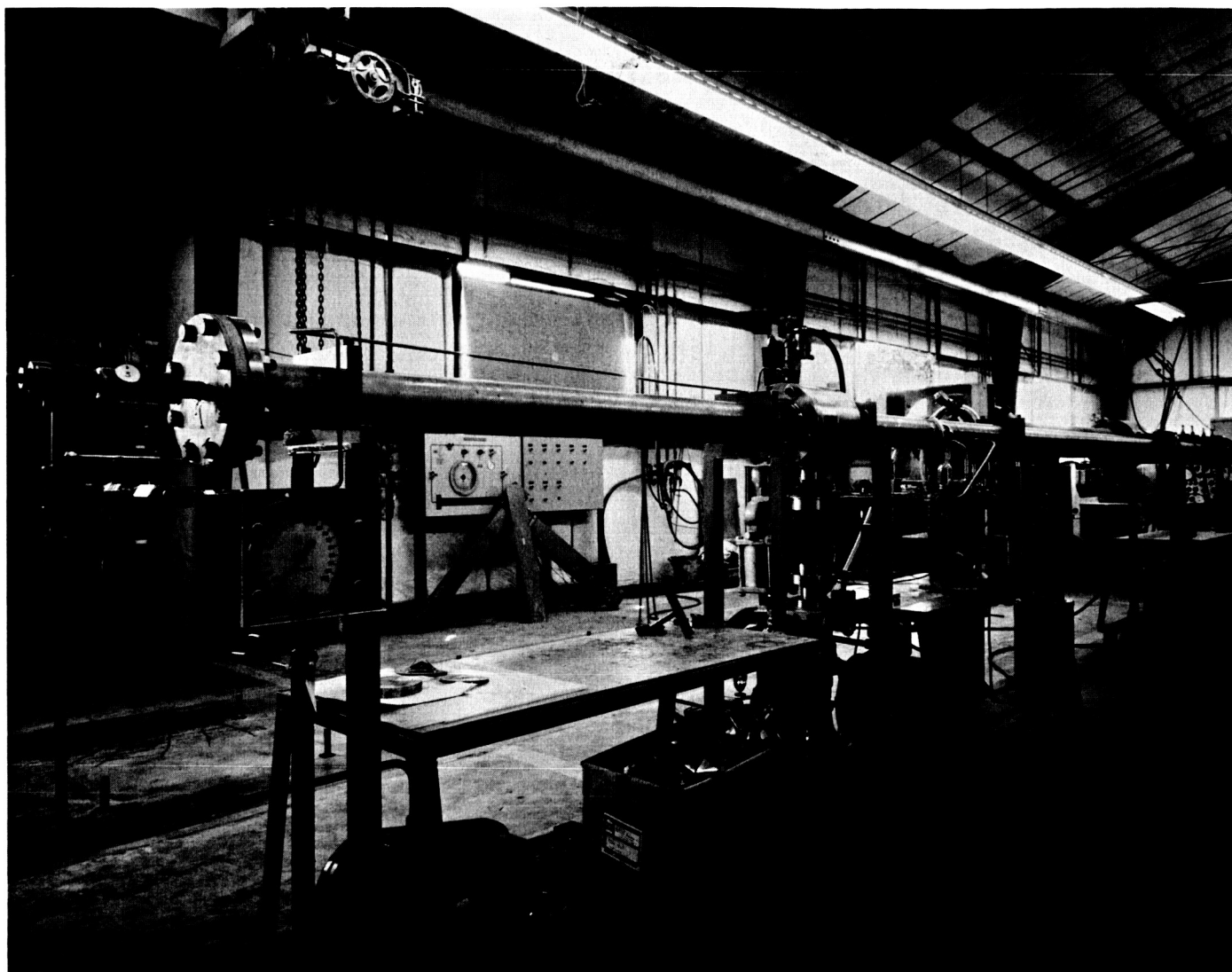
Fig. 1. Photograph of 3-in.-D shock tube
