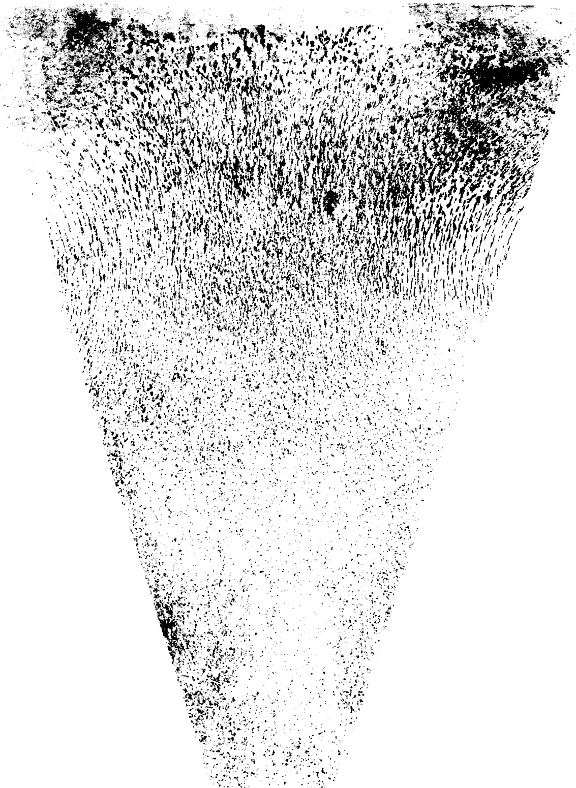
Fig. 90: Magnetic Field of the Downstream Solenoid of Figs. 73 and 74.
