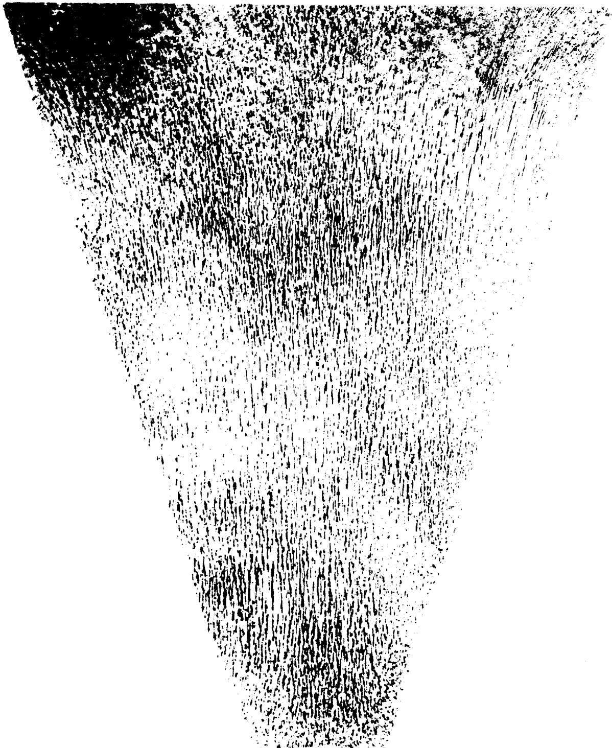
Fig. 89: Magnetic Field of Conical Coil of Figs. 73 and 74
