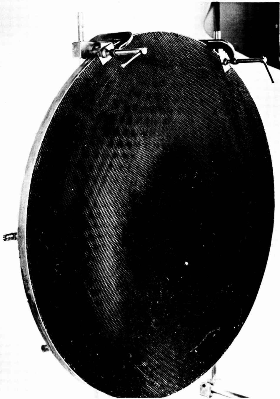
Fig. 125: The Target-Calorimeter After an Engine Run
