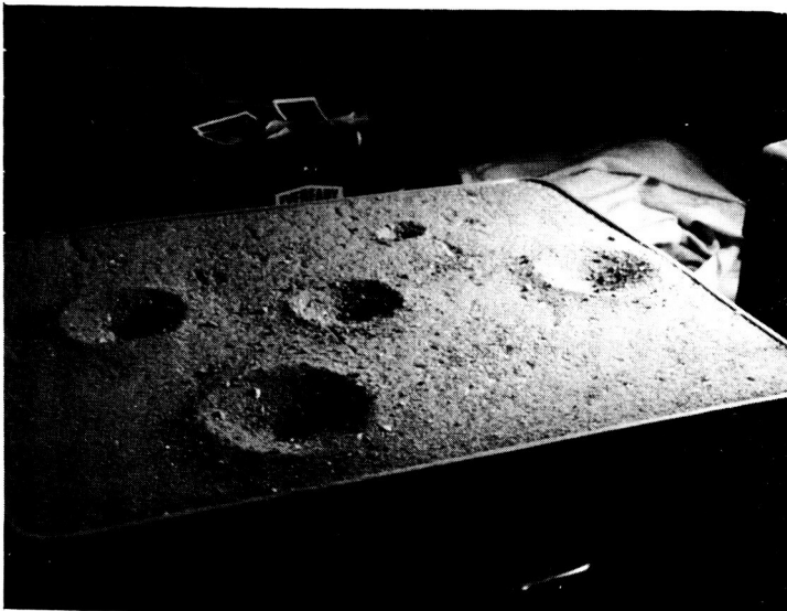
Fig. 65 CRATERS FORMED IN WELL GRADED RIVER SAND
